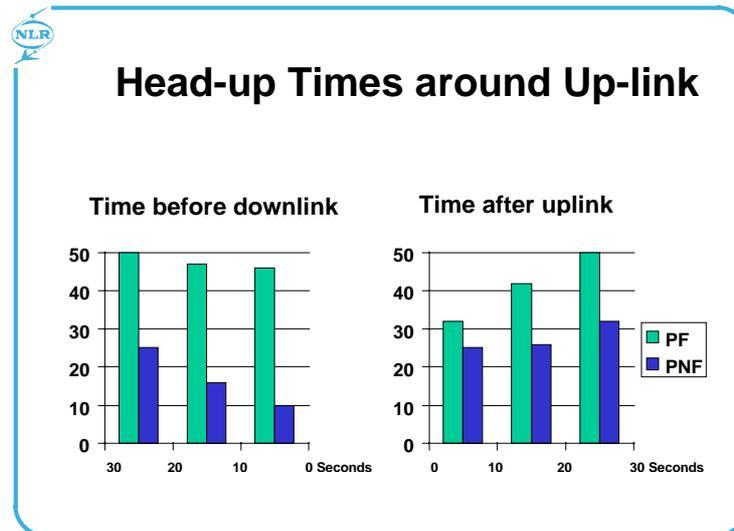
**Figure 20:** Measured percentage head up time for a Pilot Flying (PF) and Pilot Non-flying (PNF) when handling respectively a down link message and an up link message. Time 'zero' is the point where the message is sent or received respectively. Note the PF also going head down after receiving an up link.
