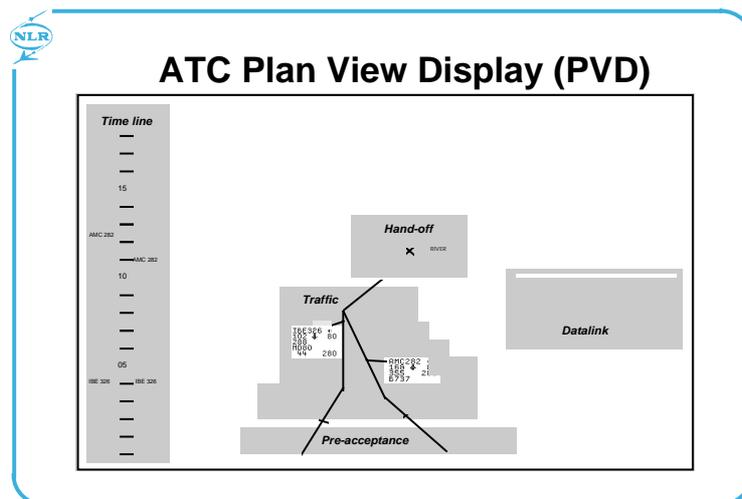
**Figure 14:** Display layout of a PVD with arrival scheduler at the left, aircraft hand-off area and datalink communication status panel. The areas are used by the POG equipment to provide area-related data on eye scans, durations, transitions, etc.
